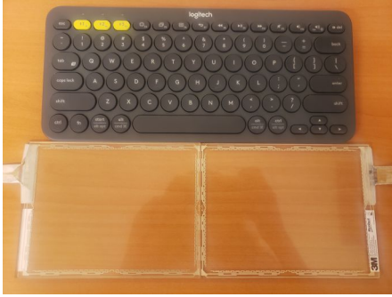
Figure 3: Sketch of electrovibrating keyboard made with an off-the-shelf keyboard and two capacitive plates.
