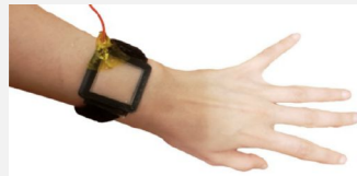
Figure 2. Sketch of electro vibrating watch with cut capacitive plates.
