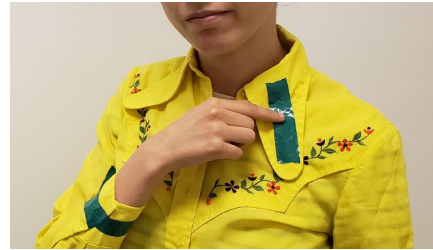
Figure 1: Mock-up of flexible electro vibrating surfaces attached to the outer surface of a collar and cuffs.
