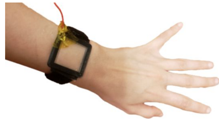
Figure 2: Sketch of electro vibrating watch with cut capacitive plates.
